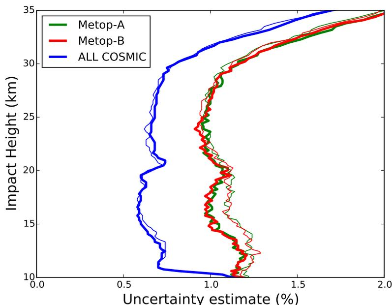
**Figure 1.3:** The estimated standard deviation of the bending angle errors for the Metop-A, Metop-B and the COSMIC radio occultation measurements in the northern hemisphere. The thick lines are for setting occultations and the thin lines are for rising occultations.
