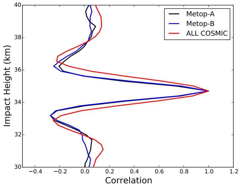
**Figure 1.7:** The bending angle error correlation estimates for setting observations near 34 km in the northern hemisphere.
