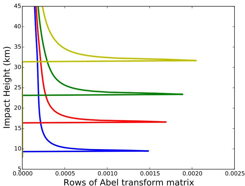
**Figure 1.11:** A selection of rows from the Abel transform matrix,  $\mathbf{A}$ . The peak value increases with height because the impact parameter separation increases.
