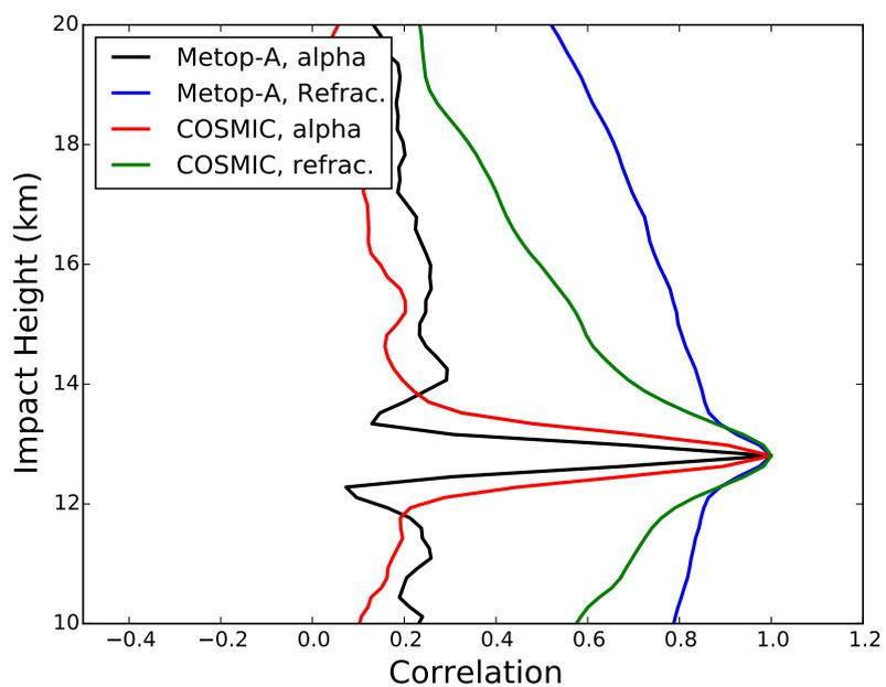
**Figure 1.15:** . The Metop-A GRAS and COSMIC bending angle and refractivity correlations near 13 km for rising occultations.
