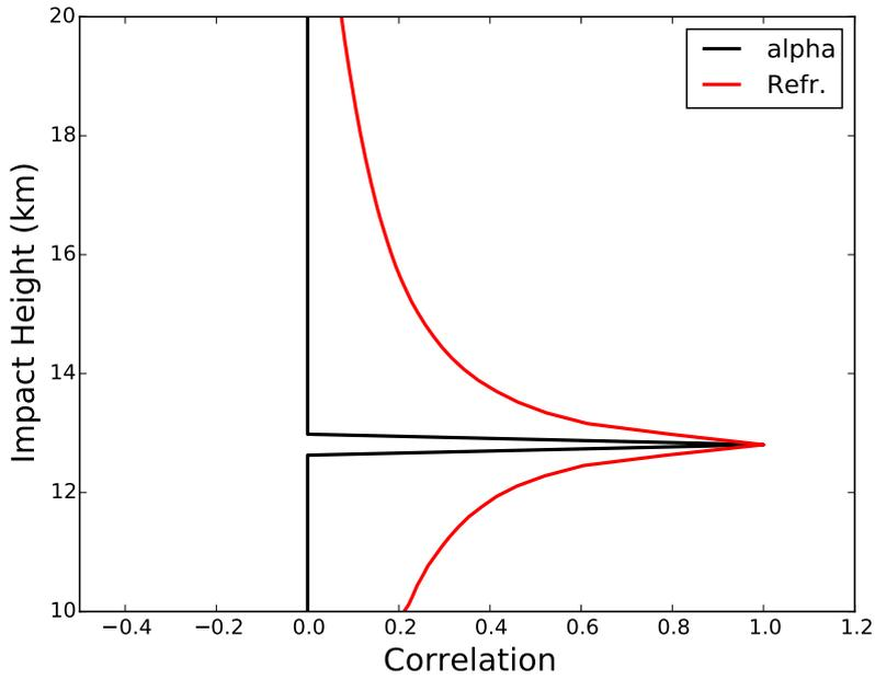
**Figure 1.13:** . The broadening of a “delta function” bending angle correlation by the Abel transform.
