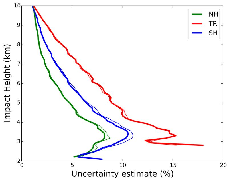
**Figure 1.8:** The bending angle error estimates in the troposphere for the COSMIC measurements. The thick lines are using a 2D observation operator and the thin lines are using a 1D observation operator.
