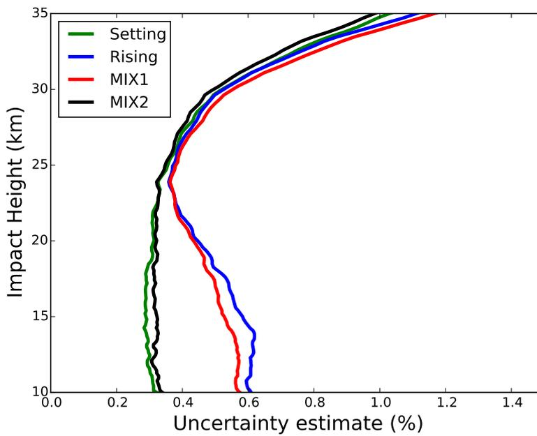
**Figure 1.10:** . The standard deviation of the refractivity errors for Metop-A rising and setting occultations. The artificial bending angle covariance matrix, MIX1, uses the bending angle standard deviations for setting measurements and the correlations from the rising occultations. Conversely the MIX2 matrix uses the standard deviations from rising occultations and correlations from setting occultations.
