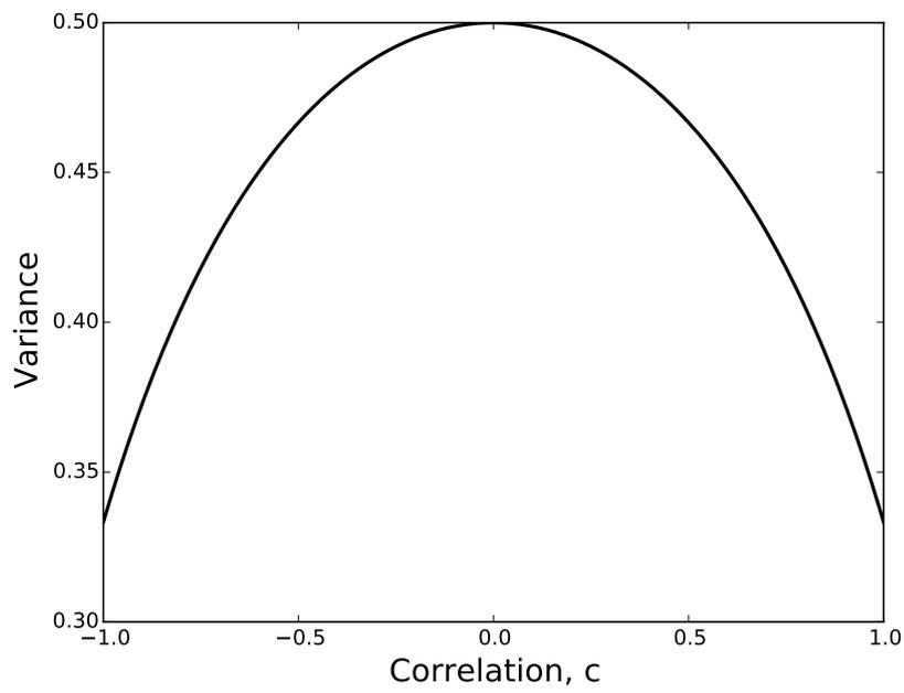
**Figure 3.1:** The variation of the solution error variance with measurement error correlation  $c$  based on Eq.3.2.
