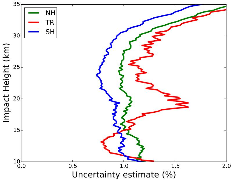
**Figure 1.1:** The standard deviation of the observation errors (uncertainty) in the NH, TR and SH for setting Metop-A GRAS measurements. The period is January 1-31, 2015, and the results are shown as a percentage of the mean bending angle profiles for each area.
