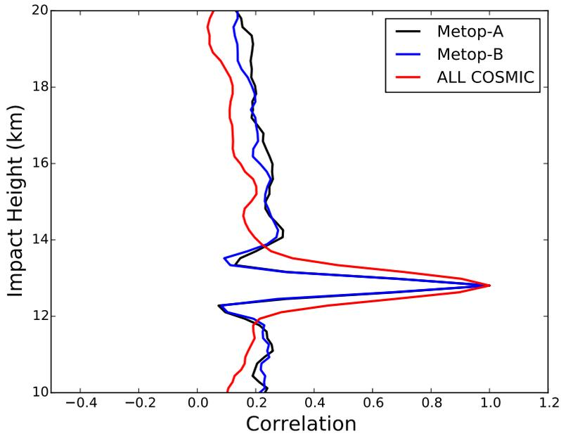
**Figure 1.5:** . The bending angle error correlation estimates for rising observations near 13 km in the northern hemisphere.
