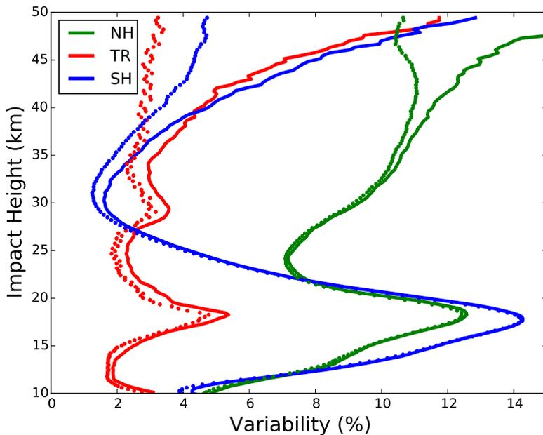
**Figure 1.2:** The observed and forward modeled bending angle variability values for the Metop-A setting measurements. The results for the observed (solid) and forward modeled (dotted) values are plotted as a percentage of the respective observed and modeled mean profiles.
