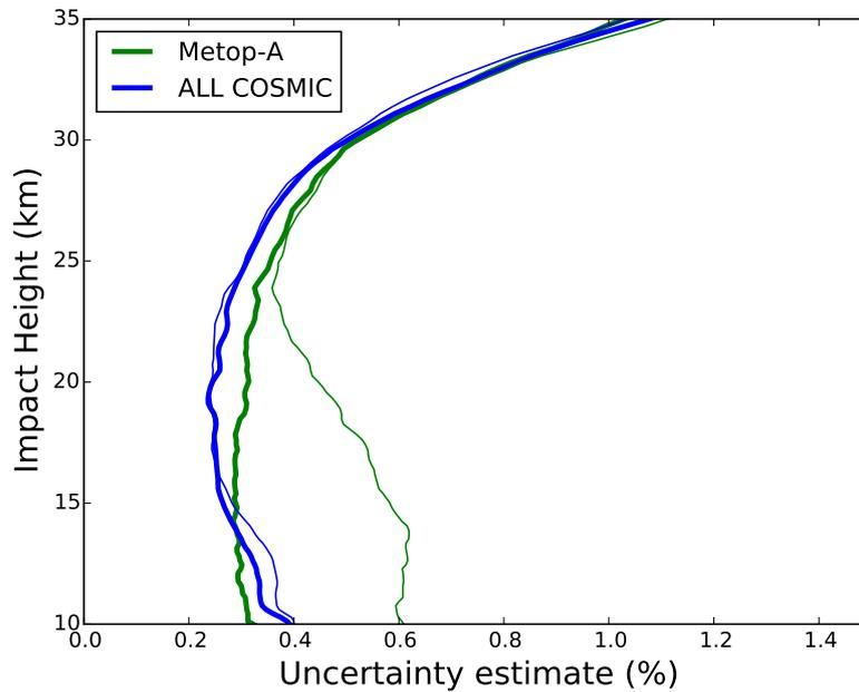
**Figure 1.9:** The standard deviation of the refractivity errors for Metop-A and the COSMIC measurements in the northern hemisphere estimated by propagating the bending angle error covariance matrix through the linearized Abel transform. Thick lines denote the setting observations and thin lines denote rising occultations.
