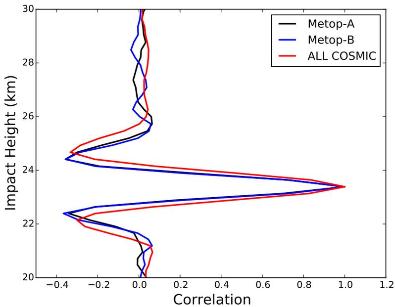
**Figure 1.6:** . The bending angle error correlation estimates for setting observations near 23 km in the northern hemisphere.
