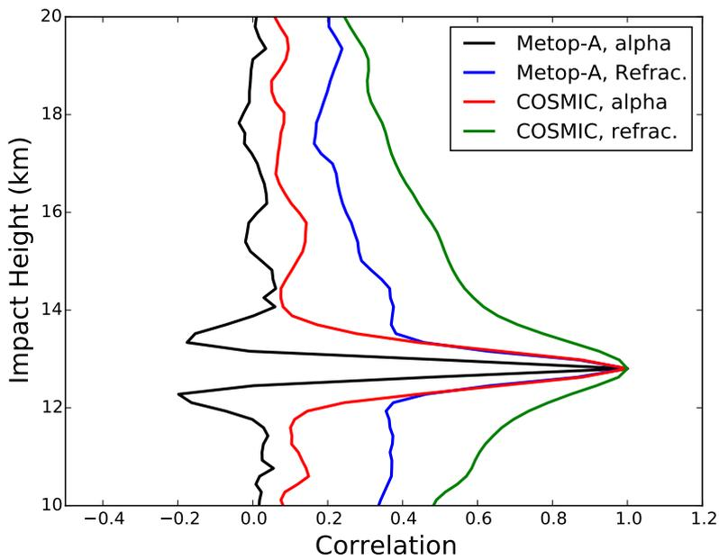
**Figure 1.14:** . The Metop-A GRAS and COSMIC bending angle and refractivity correlations near 13 km for setting occultations.
