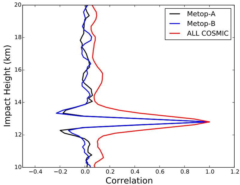
**Figure 1.4:** . The bending angle error correlation estimates for setting observations near 13 km in the northern hemisphere.
